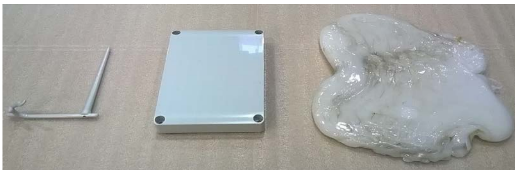
Plastic waste from left to right: Runners, Defective component, Lumps
